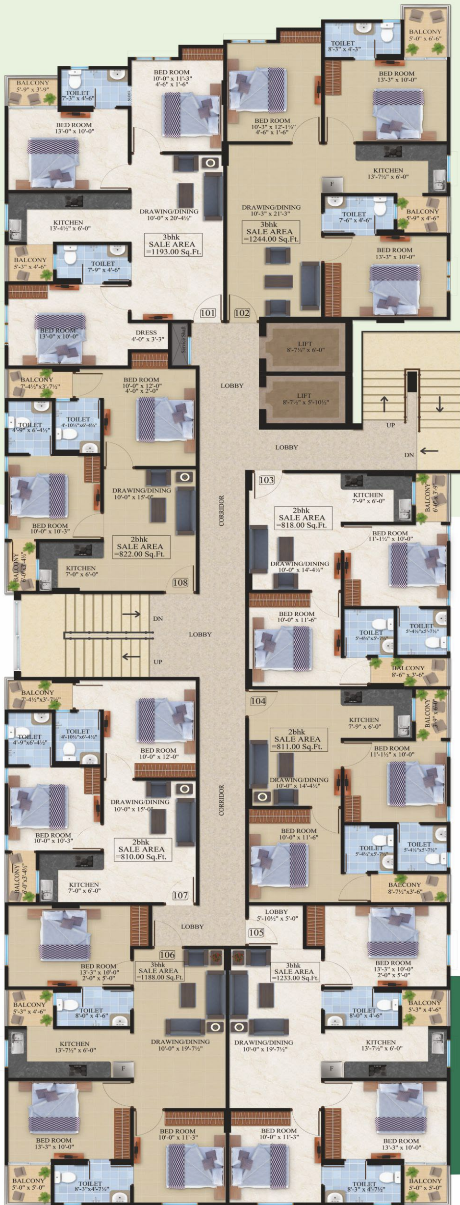
Typical Floor Plan (Ground to 6th & 8th Floor)
